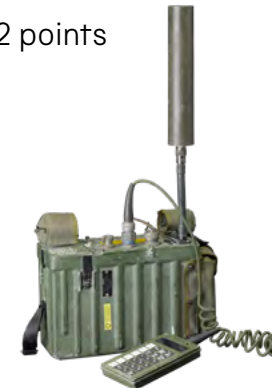
AN/PSN-8 Manpack GPS receiver
