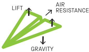
Gravity pulls everything downwards. But as they move towards the ground, the wings of the aeroplane, the wings of the glider and the blades of the helicopter create higher air pressure underneath than on top. This creates a lift force that counteracts some of gravity's pull and makes them fall more slowly. Moving through air also creates a kind of friction called air resistance, or 'drag', which tends to slow down anything moving through the air.
